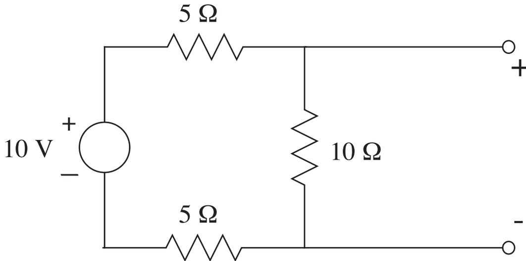
For the circuit above, the Thevenin equivalent circuit has
