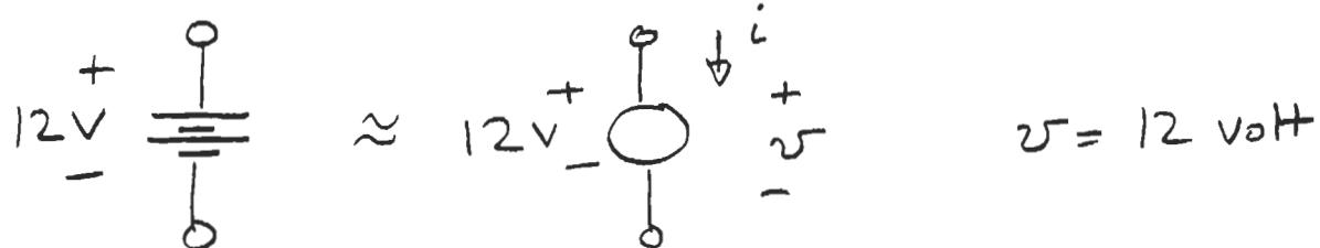
Case 2 Current is significant enough that voltage varies due to current flow.
