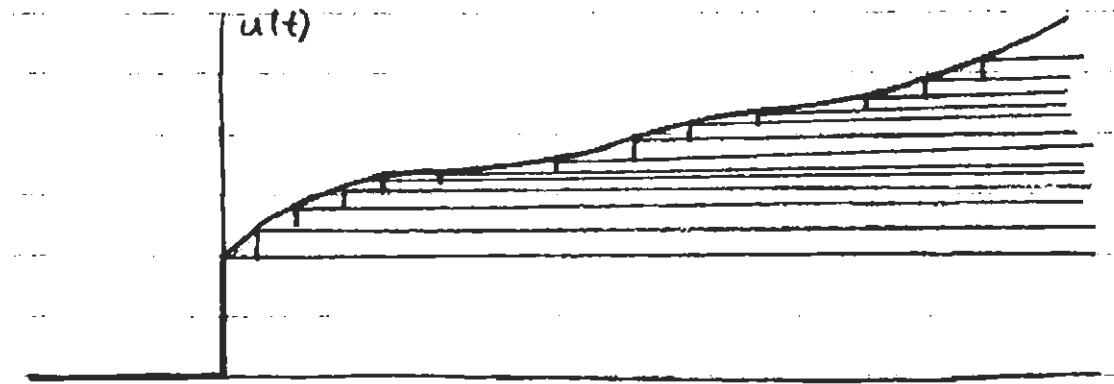
Can represent  $u(t)$  arbitrarily well by summing a series of scaled, delayed steps
