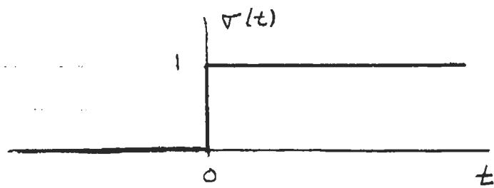
The step response of an LTI system is the output of the system when the input to the system is a unit step.
