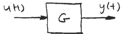
The output  $y(t)$  is a functional of the input signal  $u(t)$ :
