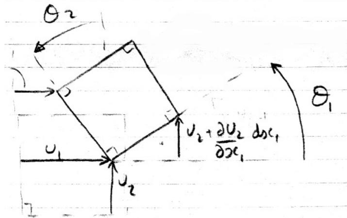
$$\theta_1 = \frac{u_2 + \frac{\partial u_2}{\partial x_1} dx_1 - u_2}{dx_1} = \frac{\partial u_2}{\partial x_1} \quad \text{as before}$$
