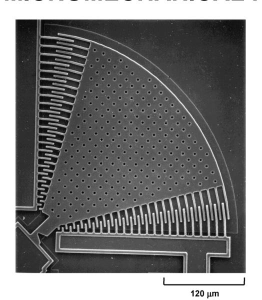
Fatigue test device (Courtesy of Stuart Brown. Used with permission.)
