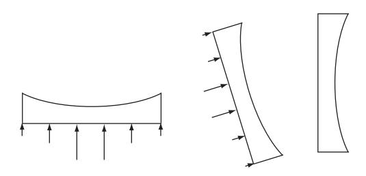
The distortion of the mirror under its own weight can be corrected by applying forces to the back surface. (Adapted from Ashby.)
