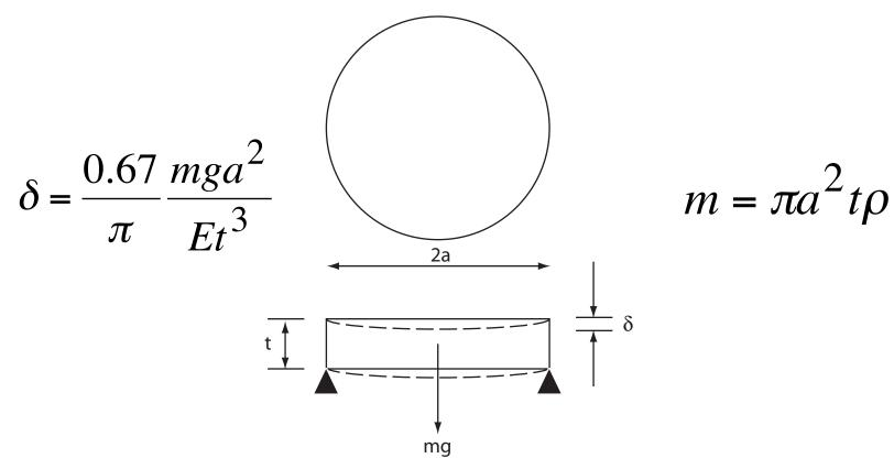
The elastic deflection of a telescope mirror (shown as a flat disc), under its own weight. (Adapted from Ashby.)
