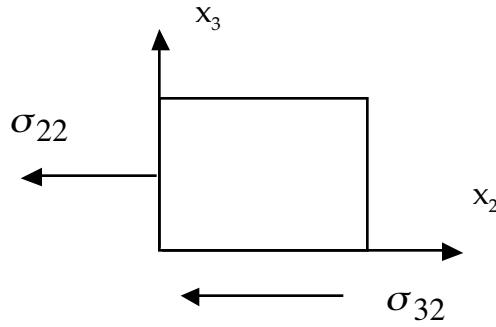
$\sigma_{22}$  acts on the negative  $x_2$  face (i.e. the face with the negative  $x_2$  direction as its normal) in the negative  $x_2$  direction. This makes it a positive (i.e tensile stress) – it is pulling out of the element. This is the same convention that we used for tensile forces in bars of trusses.
