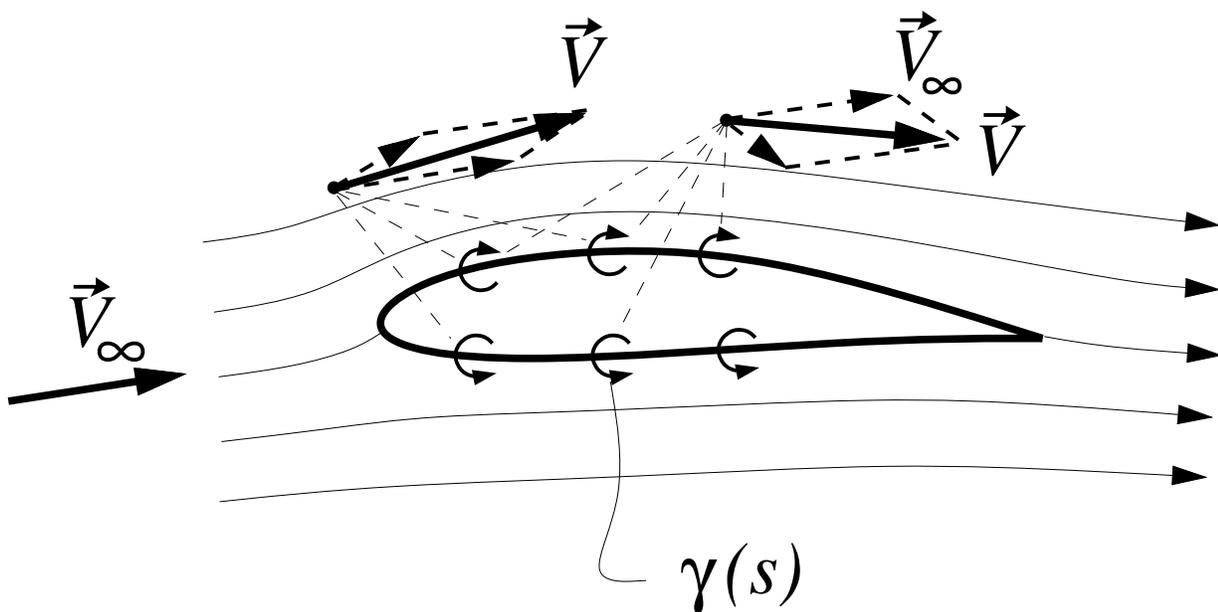
The circulation of  $\vec{V}_1(x, y)$  about the circuit of perimeter  $s_{\text{tot}}$  is  $\Gamma_1$ .
