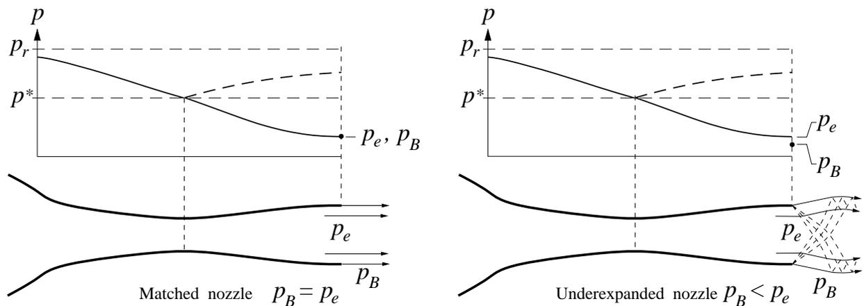
Underexpanded nozzle flow. In this case, the back pressure is reduced below the isentropic exit pressure, so that  $p_B < p_e$ . The duct nozzle flow must now expand to reach  $p_B$ , which is done through expansion fans attached to the duct nozzle edges.
