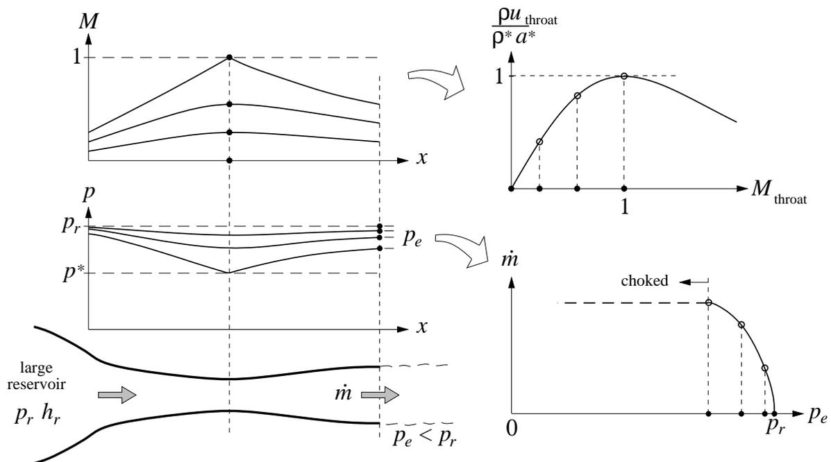
If we examine the various flow properties along the duct, it is evident that the onset of choking coincides with the *throat* reaching  $M = 1$  locally. This also corresponds to the
