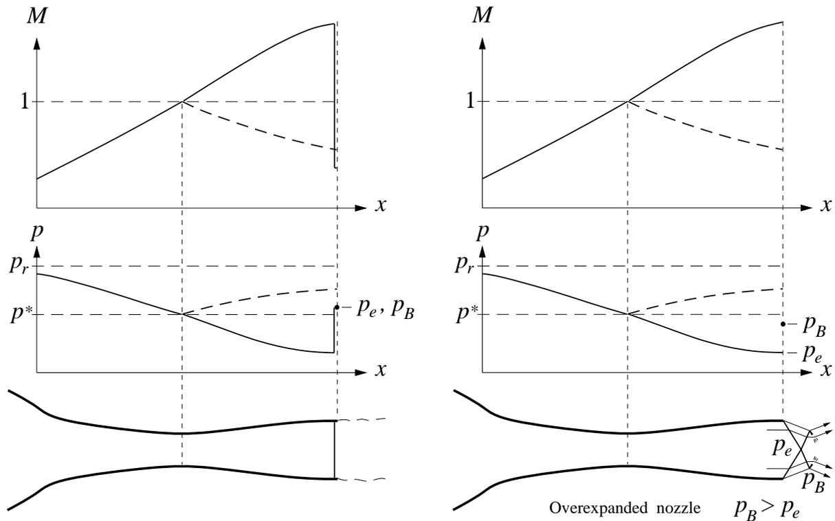
Matched nozzle flow. In this case, the back pressure is reduced further until  $p_B = p_e$ . The duct nozzle flow comes out at the same pressure as the surrounding air, and hence no turning takes place.
