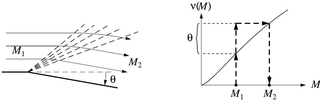
This can be considered an implicit definition of  $M_2(M_1, \theta)$ , which can be evaluated graphically using the  $\nu(M)$  function plot, as shown in the figure.
