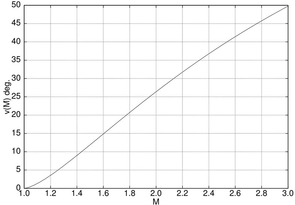
Equation (3) can be applied to any two points within an expansion fan, but the most common use is to relate the two flow conditions before and after the fan. Reverting back to our previous notation where  $\theta$  is the total turning of the corner, the relation between  $\theta$  and the upstream and downstream Mach number is
