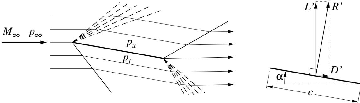
The pressure difference produces a resultant force/span  $R'$  acting normal to the plate, which can be resolved into lift and drag components.
