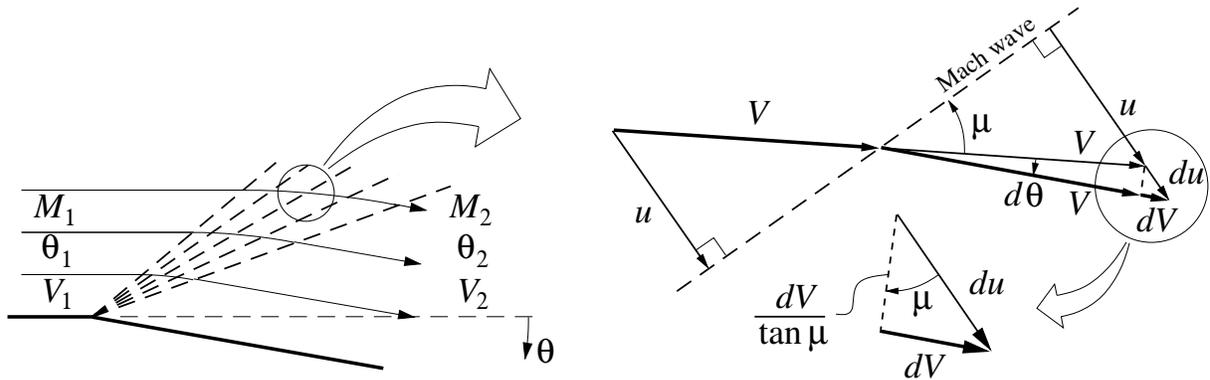
From the  $u$ - $V$  and  $du$ - $dV$  velocity triangles, it is evident that  $d\theta$  and  $dV$  are related by
