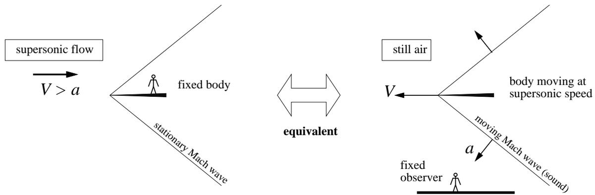
The angle  $\mu$  of a Mach wave relative to the flow direction is called the *Mach angle*. It can be determined by considering the wave to be the superposition of many pulses emitted by the body, each one producing a disturbance circle (in 2-D) or sphere (in 3-D) which expands at the speed of sound  $a$ . At some time interval  $t$  after the pulse is emitted, the radius of the circle will be  $at$ , while the body will travel a distance  $Vt$ . The Mach angle is then seen to be
