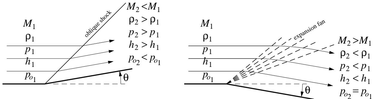
normal shock, and across an expansion fan they are in the opposite direction. One important difference is that  $p_o$  decreases across the shock, while the fan is isentropic, so that it has no loss of total pressure, and hence  $p_{o2} = p_{o1}$ .
