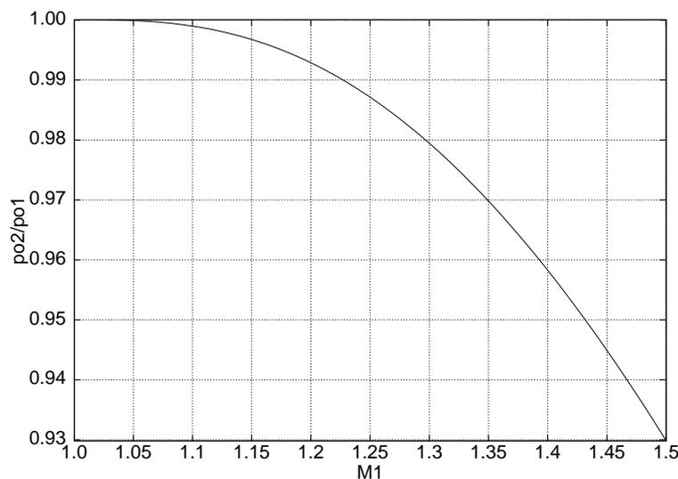
The fractional shock total-pressure loss  $1 - p_{o2}/p_{o1}$  is seen to be small for  $M_1$  close to unity, but increases rapidly for higher Mach numbers. Minimizing this loss is of great practical importance, since it cuts directly into the performance of supersonic air-breathing engines.
