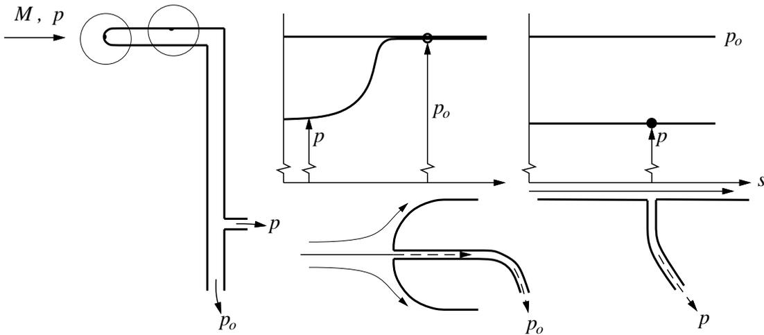
The pitot-static combination therefore constitutes a *Mach meter*. With  $M^2$  known, we can then also determine the dynamic pressure.
