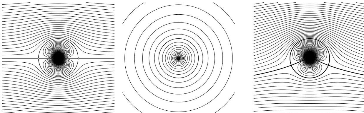
The radial and tangential velocities can be obtained by differentiating the stream function as follows.
