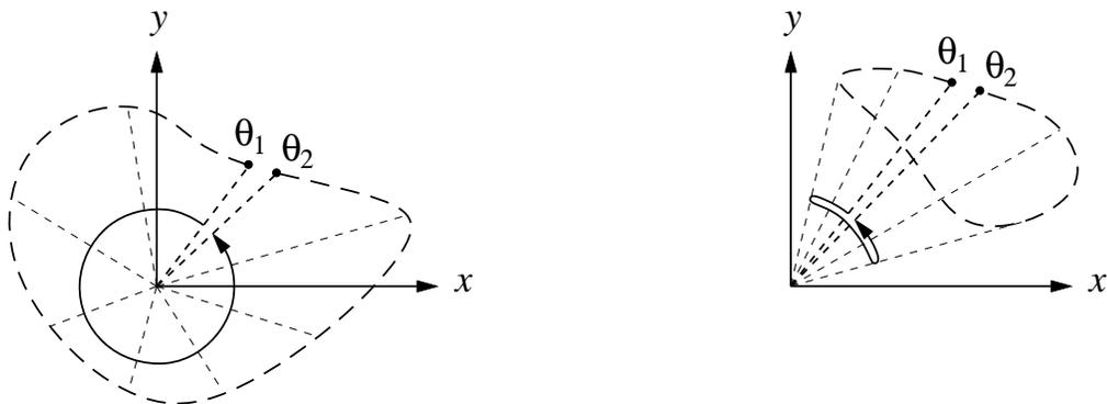
In lieu of  $C$ , it is convenient to redefine the vortex velocity field directly in terms of the circulation of any circuit which encloses the vortex origin.
