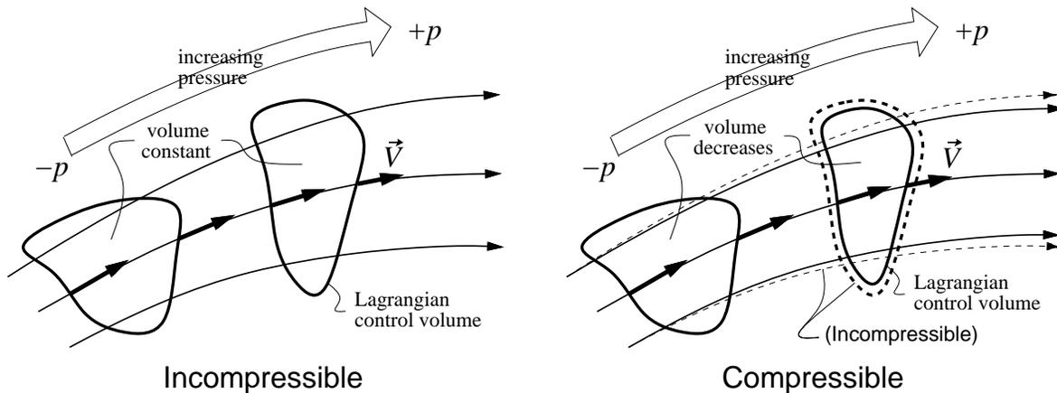
Many of the relations developed for incompressible (i.e. low speed) flows must be revisited and modified. For example, the Bernoulli equation is no longer valid,
