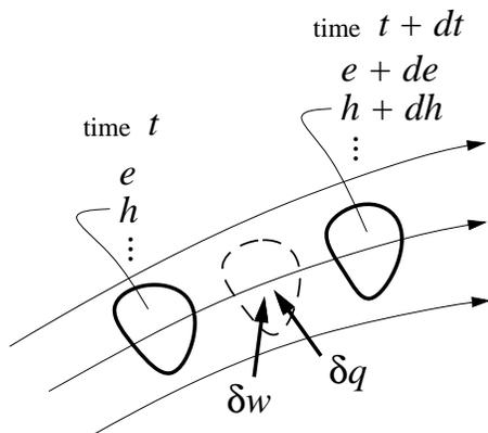
Over the short time interval  $dt$ , the CV undergoes a *process* where it receives work  $\delta w$  and heat  $\delta q$  from its surroundings, both per unit mass. This process results in changes in the state of the CV, described by the increments  $de$ ,  $dh$ ,  $dp \dots$ . The first law of thermodynamics for the process is
