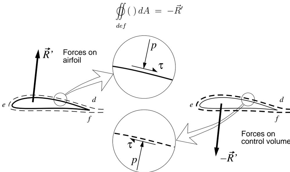
An intuitive explanation is that the aerodynamic force exerted by the fluid on the body is exactly equal and opposite to the force which the body exerts on the fluid.
