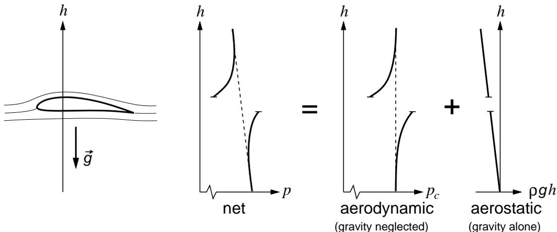
For clarity, we will from now on refer to  $p_c$  simply as  $p$ . The understanding is that the forces and moments computed using this  $p$  will not include the contributions of buoyancy. However, buoyancy is relatively easy to compute, and can be added as a secondary step if appropriate. It should be noted that buoyancy is rarely significant in aerodynamic flow situations, one exception being lighter-than-air vehicles like blimps.
