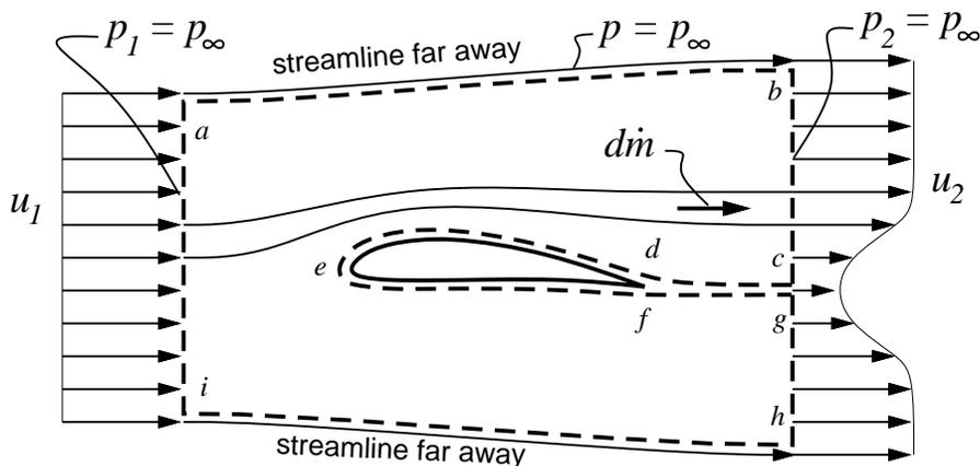
The surface integrals are now broken up into the individual pieces: the outermost part  $abhi$ , the body surface  $def$ , and the “cut” surfaces  $cd$  and  $fg$ .
