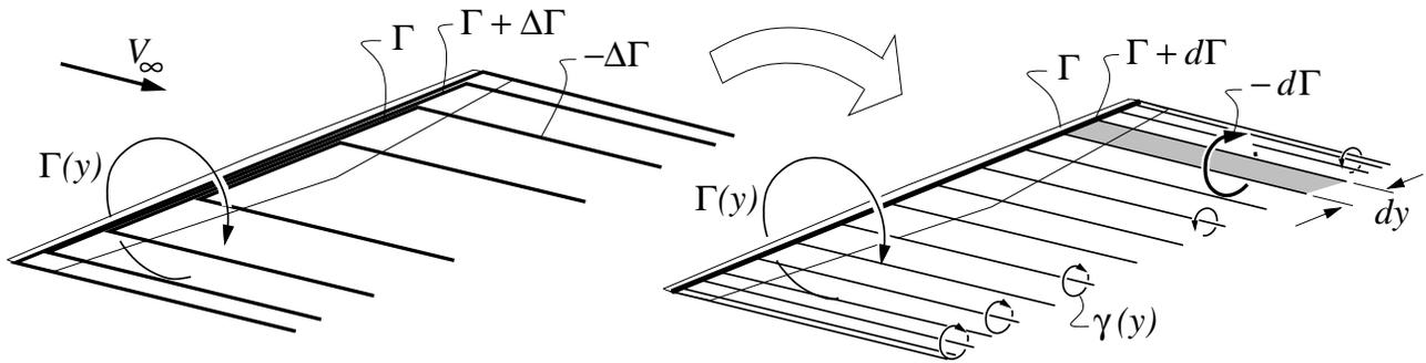
considering a small change of circulation  $d\Gamma$  between spanwise stations  $y$  and  $y + dy$ . By Helmholtz's theorem, the  $dy$ -wide sheet strip trailing between those two stations must have a circulation  $-d\Gamma$ . This then gives the local sheet strength  $\gamma(y)$ .
