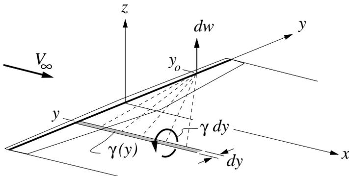
Integrating over all the wake strips gives the overall vertical velocity distribution of the whole trailing sheet.
