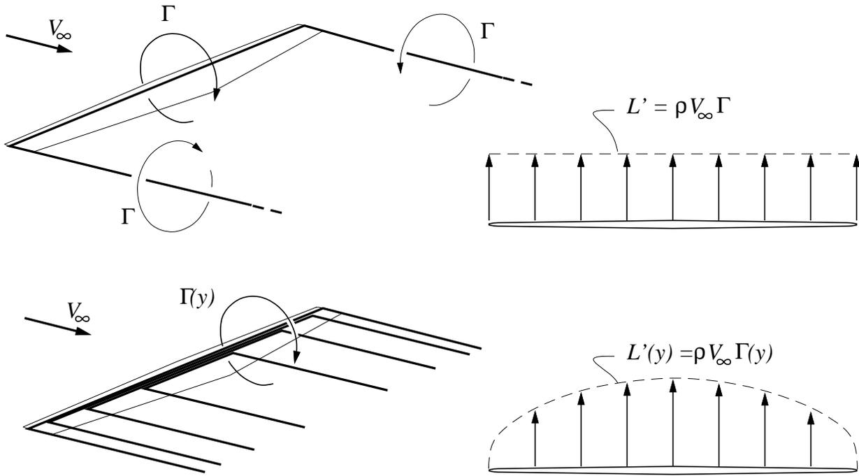
The figure shows only a few horseshoe vortices on the wing, but one can conceptually subdivide these into more and more vortices of decreasing strength, which in the limit become a *trailing vortex sheet* with strength  $\gamma(y)$ . The strength of the sheet can be determined by
