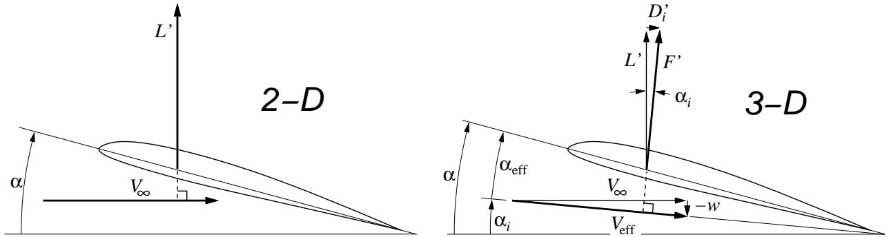
Because  $\alpha_{\text{eff}} < \alpha$ , the lift generated by the 3-D wing is less than if the downwash and induced angle were absent, as in the 2-D case. In practice, this means that the 3-D wing has to operate at a greater geometric  $\alpha$  to achieve the same lift/span as the 2-D wing.
