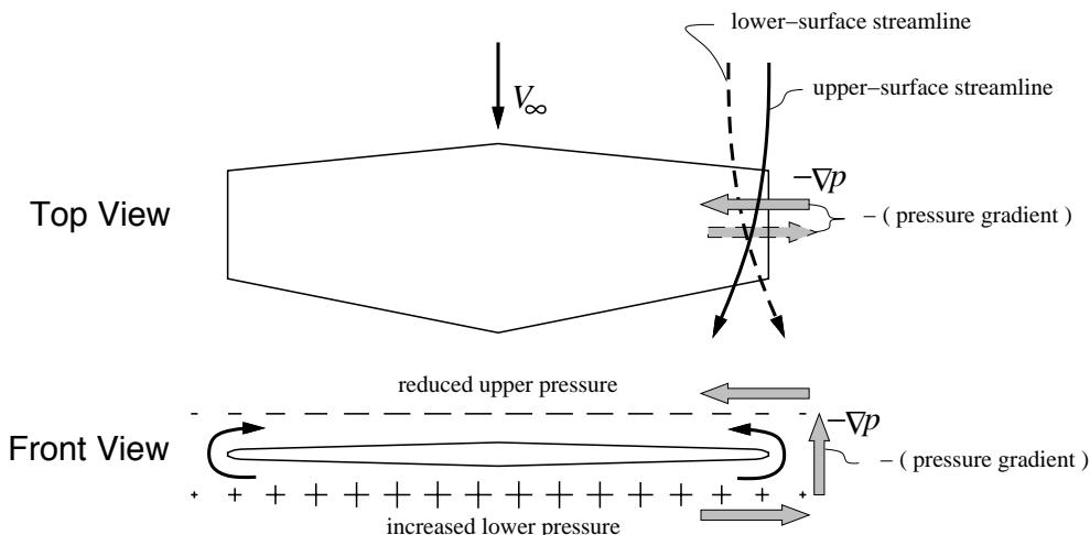
Trailing vortices. The flow curling around the tip forms a *tip vortex*, which then trails downstream, and can be easily made visible with smoke visualization.
