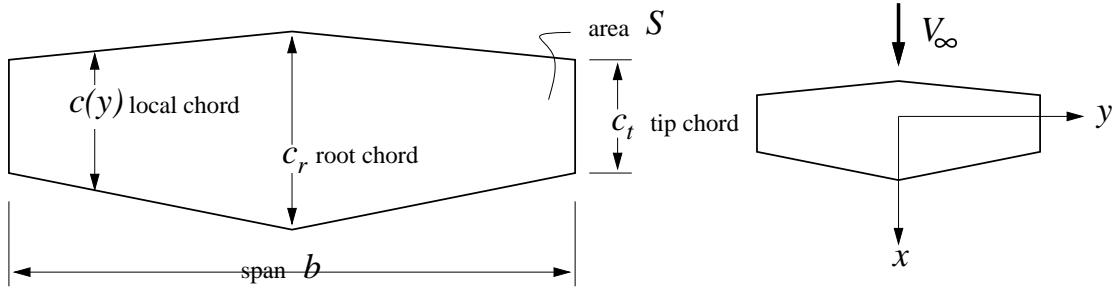
Several other relevant geometric parameters can be defined. One is the *average chord*  $c_{\text{avg}}$ , which is a simple average of the local chord  $c(y)$ .
