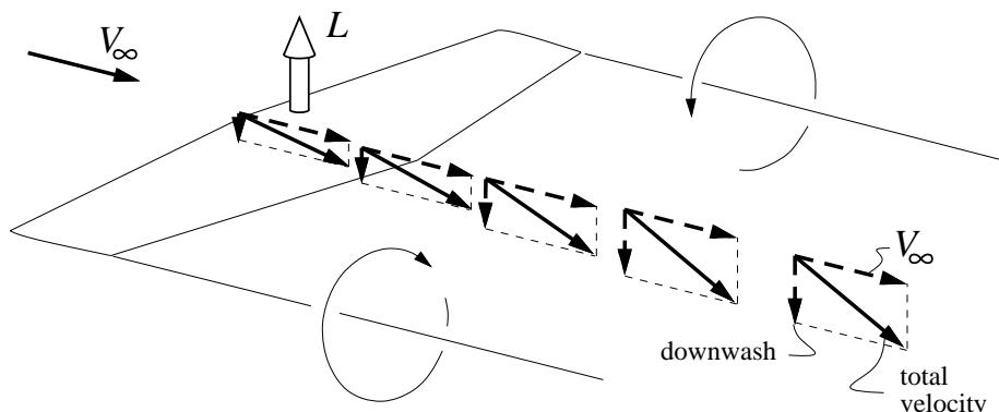
Induced angle and lift reduction. There is a nonzero downwash velocity  $-w$  at the wing itself ( $w$  is positive up). In other words, the wing operates in its own downwash. The apparent freestream velocity which the wing sees is therefore tilted by the *induced angle*
