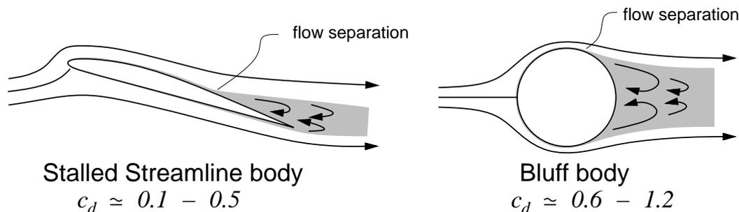
Bodies with separation exhibit much larger drag forces than comparably-sized streamline bodies without separation. When an airfoil stalls, its drag will typically increase by a factor
