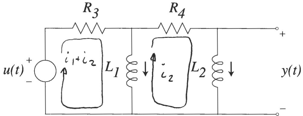
Find the differential equations that describe the input-output behavior of the circuit above, in state-space form,
