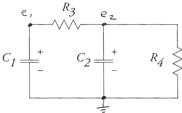
For the circuit above, find  $v_1(t)$  and  $v_2(t)$ , for the initial conditions
