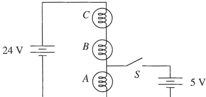
A circuit consists of three identical light bulbs, two batteries, and a switch, as shown above. When the switch  $S$  is closed, do the following increase, decrease, or stay the same? Circle one for each part.
