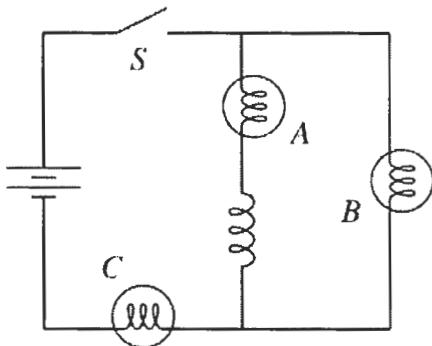
Consider the circuit above with three identical light bulbs, a battery, an inductor, and a switch. Initially, the switch is open, and has been open for a long time. The switch is then closed.
