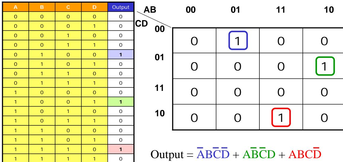
$$\text{Output} = \bar{A}\bar{B}\bar{C}\bar{D} + A\bar{B}\bar{C}D + ABC\bar{D}$$
