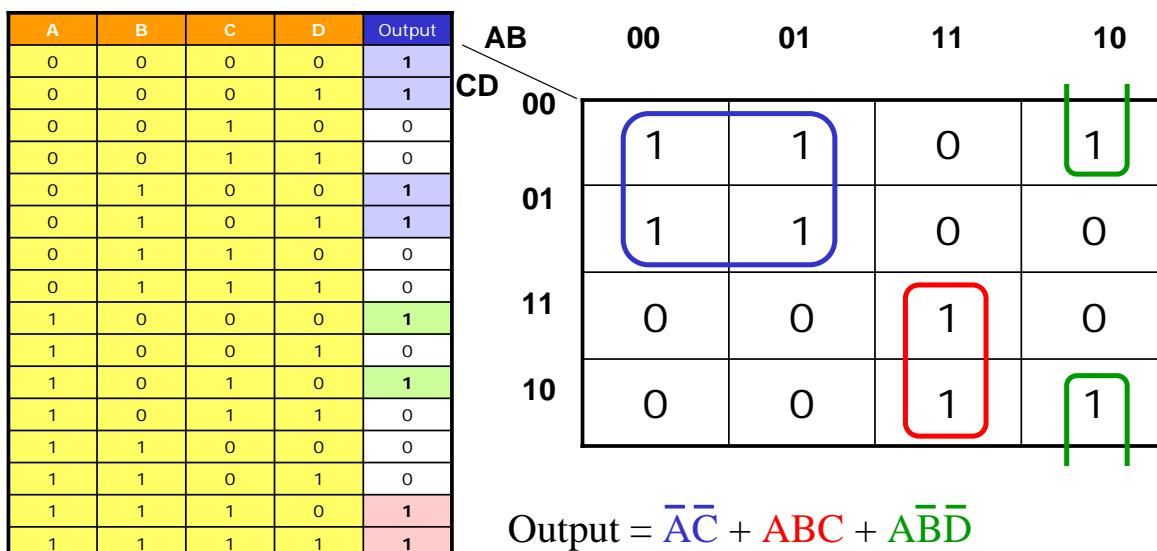
$$\text{Output} = \bar{A}\bar{C} + ABC + A\bar{B}\bar{D}$$
