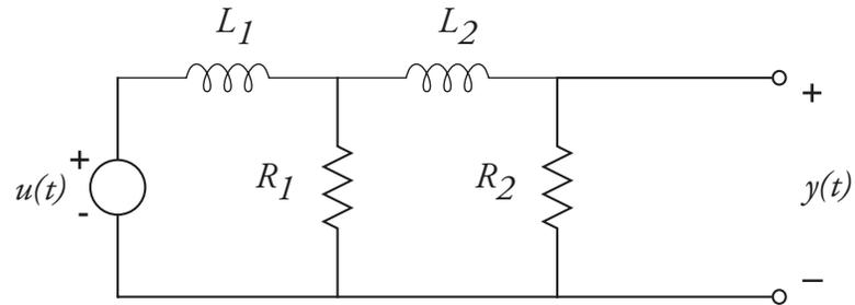
where  $L_1 = L_2 = 2$  H,  $R_1 = 2$   $\Omega$ , and  $R_2 = 3$   $\Omega$ .
