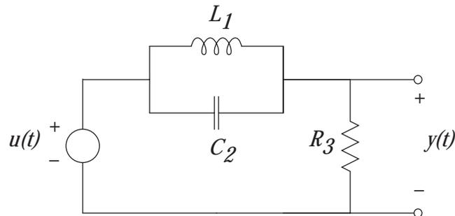
This circuit is a *notch filter*, meaning that the output  $y(t)$  is almost the same as the input  $u(t)$ , except that the circuit “filters out” frequencies in a narrow range, determined by the component values. For example, this circuit might be used to filter out 60 Hz noise caused by electrical wiring from the input to an audio system, to prevent 60 Hz “hum.”
