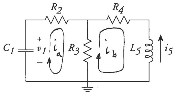
$$i_a : (R_2 + R_3)i_a - R_3 i_b - v_1 = 0$$
