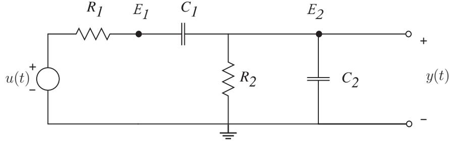
Again, use impedance methods, using the node labelling above. Then the node equations are
