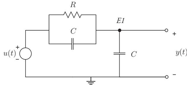
We can use impedance methods to solve for  $Y(s)$  in terms of  $U(s)$ . Label ground and  $E_1$  as shown. Then KCL at  $E_1$  yields
