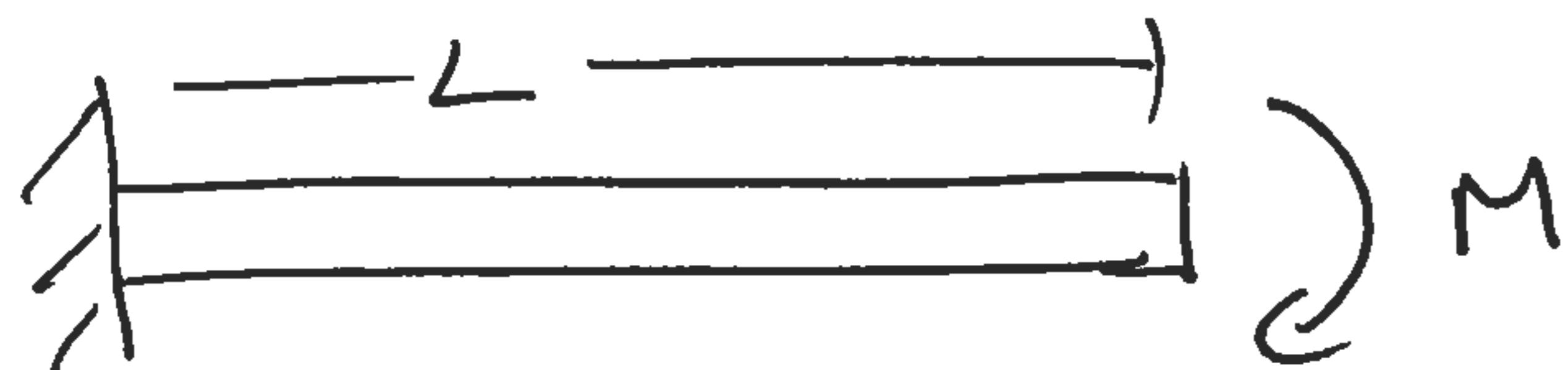
$$M22 \quad \delta = \frac{2ML^2}{\pi R^4 E} \quad \text{mass, } m = \rho \pi R^2 L$$
