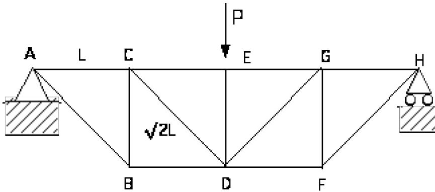
Since this is the truss that you are experimenting with in the truss lab, you can also compare the results of the experiments to the analysis. By assuming values for L, A and E (70 GPa for aluminum, 210 GPa for steel) estimate the relationship between applied load and the deflection of point D for the experimental truss and compare with your data. If the two results are not similar, suggest potential reasons for the discrepancy.
